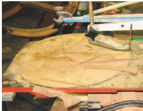
The Hegner scrollsaw is precise enough to trust with pricey veneers
